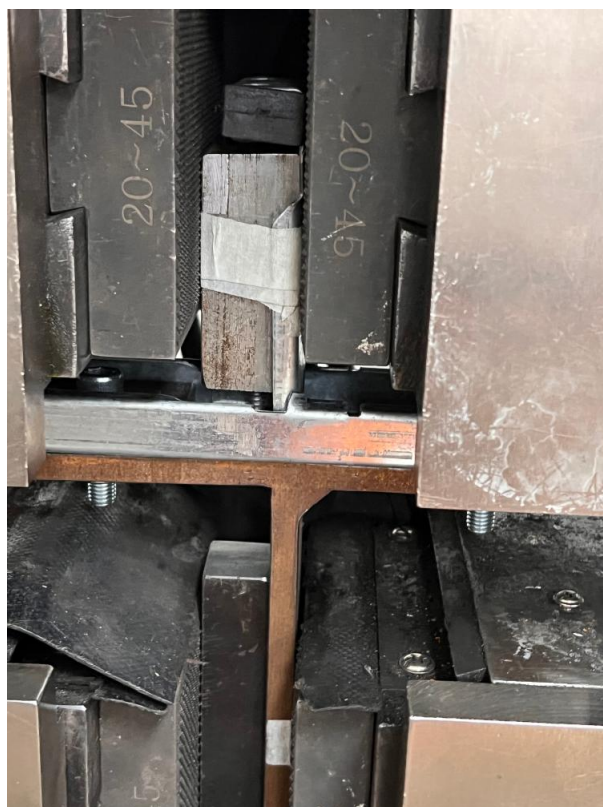
Image 4 of 4 - Failure location at ultimate load
